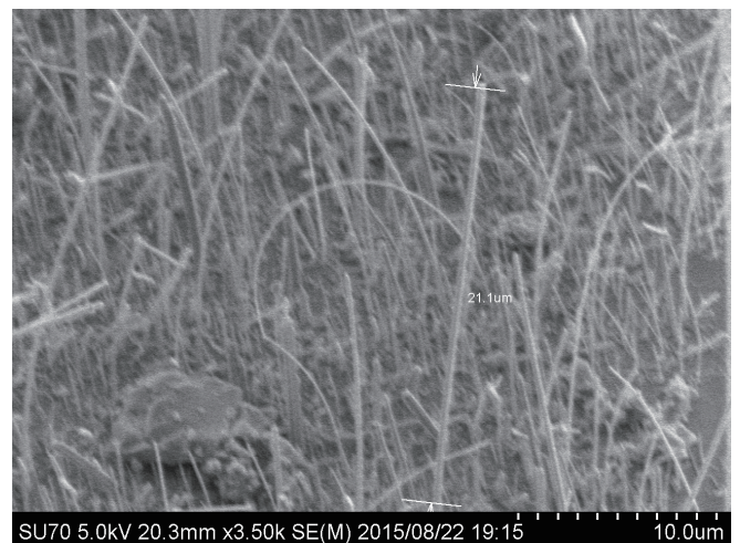
Fig. 4 Nanowires Grown by HVPE, the Stage in SEM is Titled by 40°.
